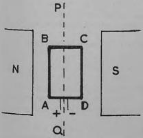
The diagram shows a rectangular coil of wire, ABCD, with AB = 3cm. and BC = 2cm., which is free to turn about the axis PQ and which is lying in a uniform magnetic field strength 20 gauss. If there are 15 turns of wire in the coil and a current of 0.1 amp. is flowing in the direction ABCD, find the magnitude and direction of the forces on AB and CD when the coil is (i) in the plane of the paper, (ii) at right-angles to the plane of the paper. What is
