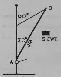
The diagram represents a jib crane with a windlass at A for hoisting the load. The rope from the windlass is parallel to the jib. Find graphically or otherwise the force exerted by the jib at B assuming the tension in the rope holding the load is the same throughout its length.
