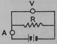
In the circuit shown in the diagram the resistances of the voltmeter V, the resistor R and the ammeter A are 1,000 ohms, 200 ohms, and 2.5 ohms respectively. The battery has an e.m.f. of 4.4 volts and a negligible internal resistance. Calculate the readings which should appear on the voltmeter and the ammeter, assuming that the voltmeter can be read to the nearest tenth of a volt
