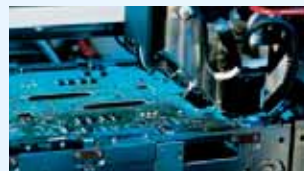
SMD insertion with automatic visual check
