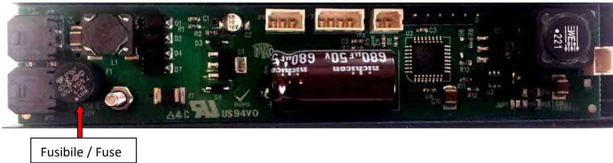
Electric circuit in rear arm
