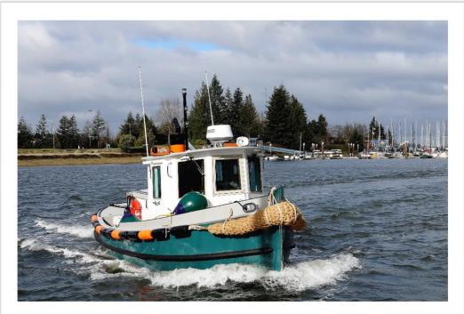
TugZilla 26, a 8 knot (top speed), 6.5 knot cruiser with a Single 110 hp. Yanmar inboard, keel drive.
