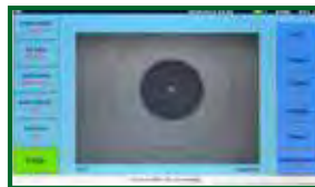
IEC 61300-3-35 Connector Inspection
