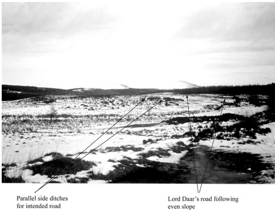
Figure 9. View at Point C on Figure 6., under light snow, showing parallel ditches
