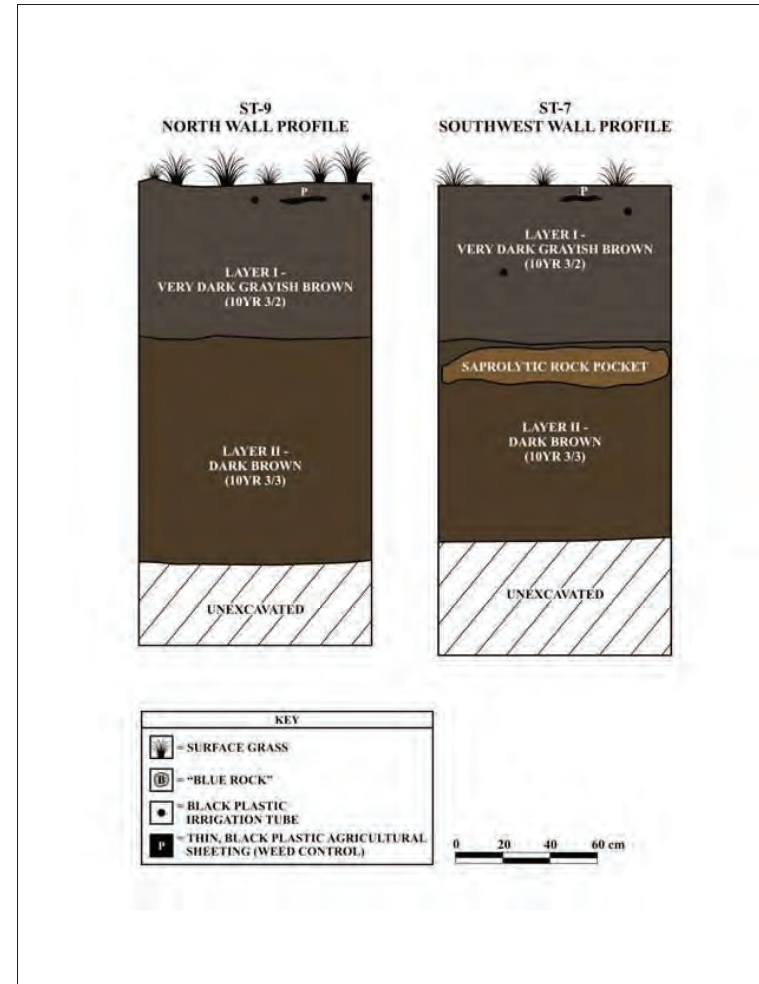
Figure 22: ST-9 and ST-7 Profiles Display Typical Subsurface Stratigraphy within Project Area.
