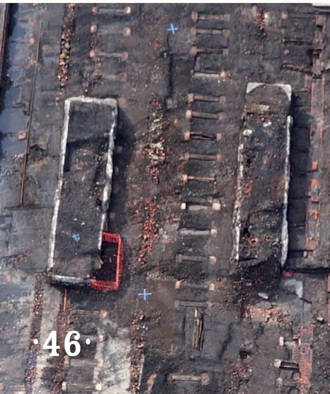
Aerial view of two of the concrete-walled air raid shelters that were set into the track bed of the travelling crane
