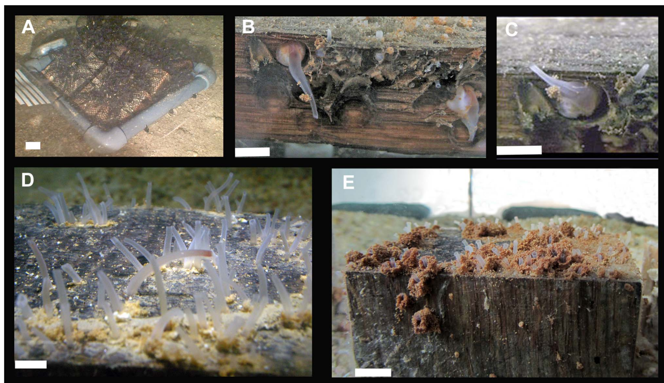
Figure 2. Experimental wood samples: A) on the seafloor at LFC at 130 m depth before recovery (artificially lit by ROV); B), C) Individuals of X. dorsalis in the aquarium in wood that was recovered after 10 months from 130 m deep in LFC; D) Xylophaga spp. the day after recovery from La Fonera Canyon (1100 m deep) in wood after 6 months immersion; E) oak from La Fonera Canyon 1100 m one week after recovery. Note the development of fecal chimneys around the siphons. doi:10.1371/journal.pone.0102887.g002
