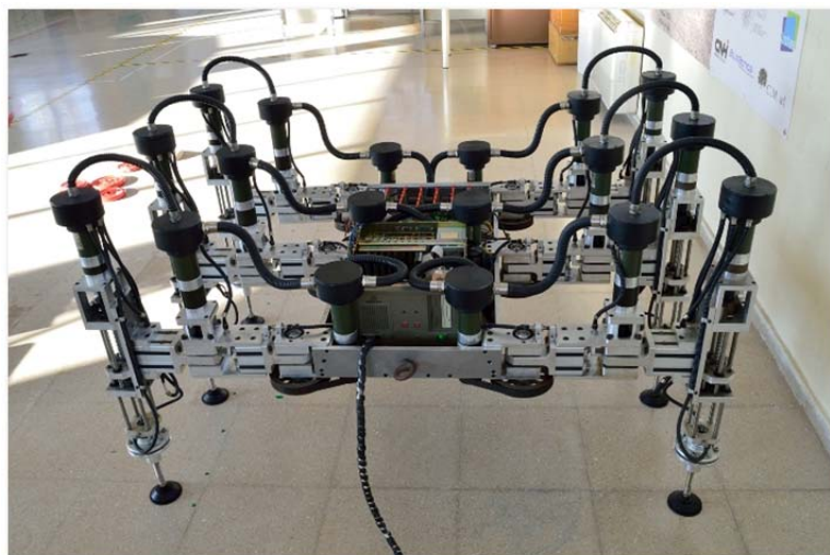
Figure 4. Hexapod walking robot in CAR (CSIC-UPM) lab.
