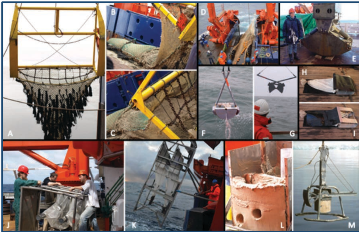
Figure 2.1.- Different gears used to collect studied material. A-C , Agassiz trawl: A , front view; B , on deck; C , catching. D , Bottom trawl. E , TV grab. F-G , Van Veen grab: F , closed; G , opened. H-I , Rauschert dredge: H , lateral view with upper rubber mat unfolded; I , lateral view with rubber mat folding over to protect the nets. J-K , Epibenthic sledge: J , setting up; K , lateral view. L-M , Giant box corer: L , catching; M , lateral view.
