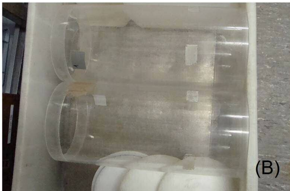
FIGURE B.4: A) A lid with different holes used to introduce the stirrer, sensors for digital records or pipettes for the Winkler titration; B) The perspex chambers ( d = 30 cm). All material provided by the Ecosystem studies department of the NIOZ-Yerseke.
