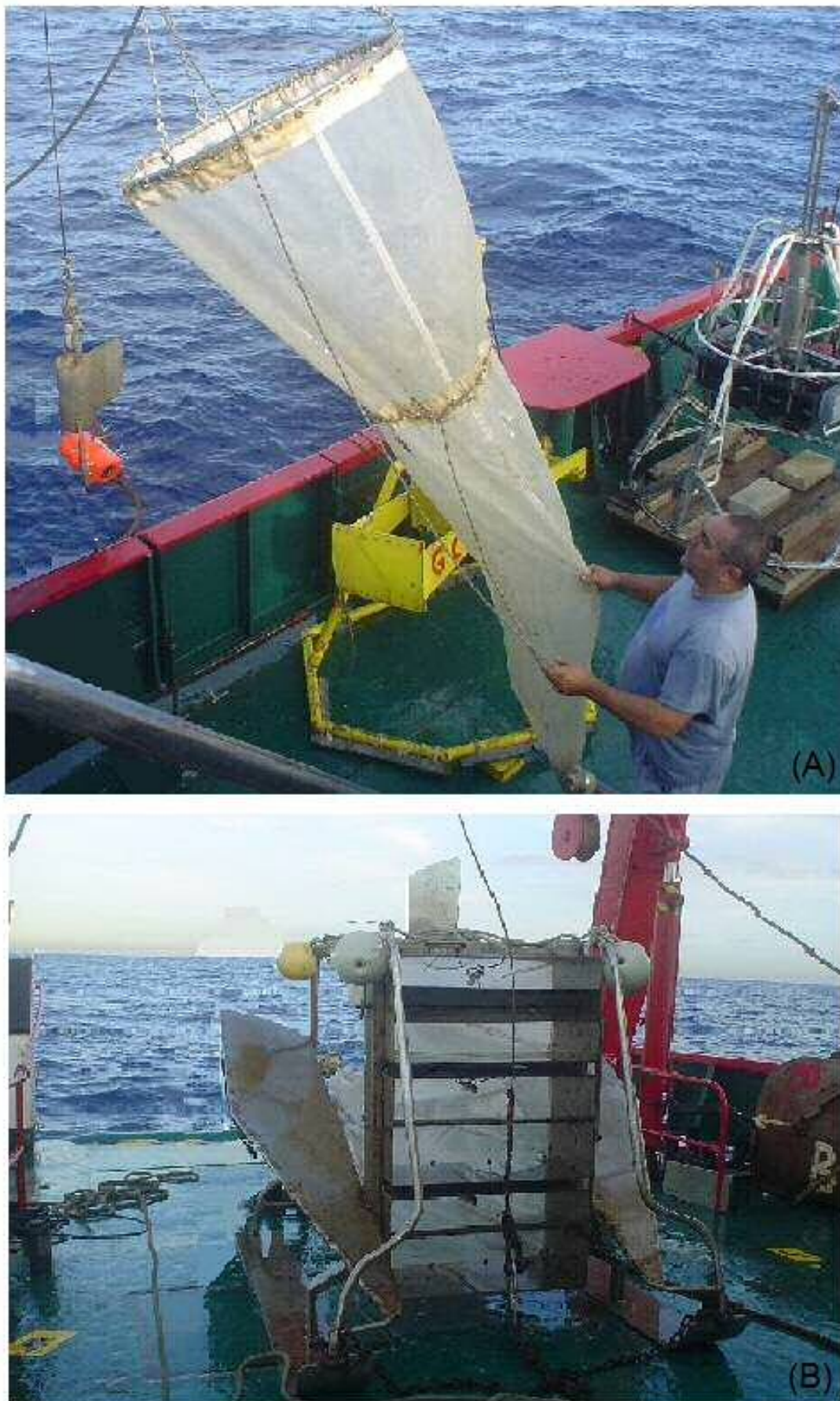
FIGURE B.3: (A) WP2 used to sample zooplankton and micronekton. (B) Suprabenthic sledge used to sample suprabenthos. B/O García del Cid, Catalan Sea, BIOMARE October, 2007.
