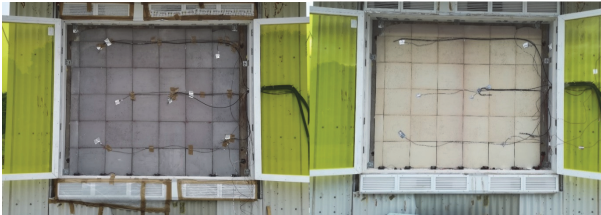
Figure 10: Detail of the thermochromic tiles in (2) high absorbance and (3) high reflectance mode
