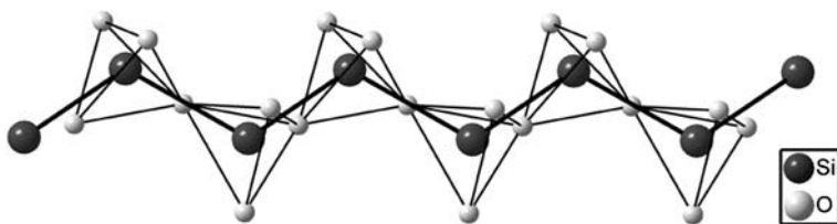
Fig. 10 The structure of an unbranched single chain anion existing in \text{Na}_4\{\text{uB}, 2, 1^1_\infty\}[\text{Si}_2\text{O}_6] , to show its similarity with the chains of fibrous sulfur and with the asbestos-like \text{SO}_3 oxide
