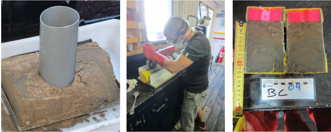
Figure 4: Left) Mini corer inserted in a BC sample. Middle) Cutting the mini corer in two halves using an electrical saw. Right) Resulting two halves of a mini core.
