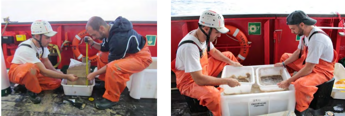
Figure 3: Left ) Taking notes of a sediment sample collected with Box-corer in the Gazul mud volcano. Right ) Sieving the 0-5 cm fraction of a sediment sample on a mesh size of 0.5 mm.
