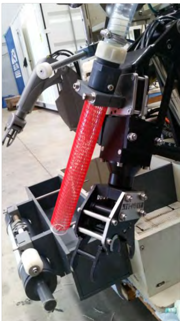
Figure 4: Suction tube installed in one of the hydraulic arms of the ROV Liropus.
