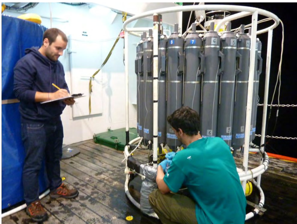
Figure 5: member of the physical and biogeochemical oceanography teams sampling the CTD-Rosette during the first leg of MEDWAVES.
