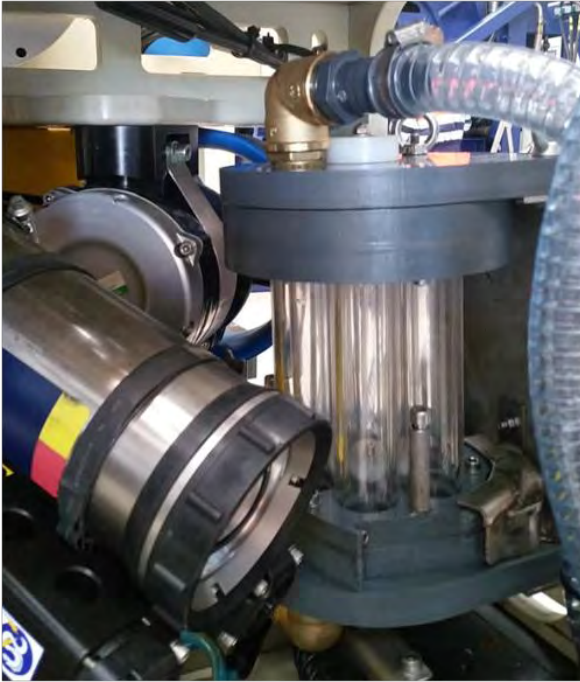
Figure 5: Step by step rotation gear and connection of the suction hose to the upper part of the sample collector.
