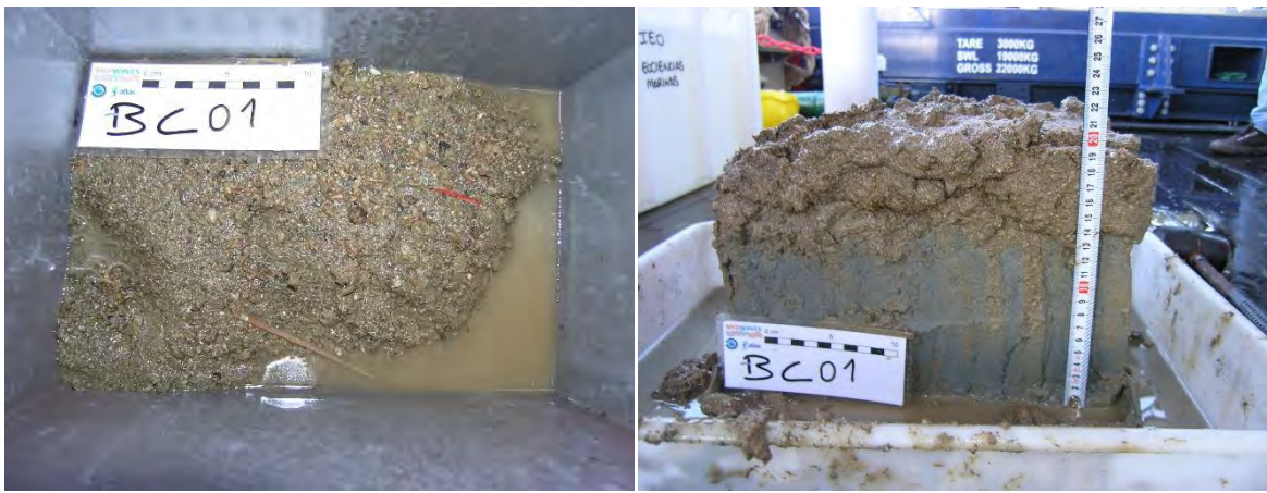
Figure 2: General view ( left ) and vertical profile ( right ) of the first sediment sample collected with the Box-corer (code: BC01) during Medwaves (Gazul MV).
