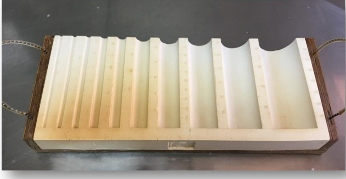
Fig. 1.3.2.3 Trophometer used on board for stomach sampling.
