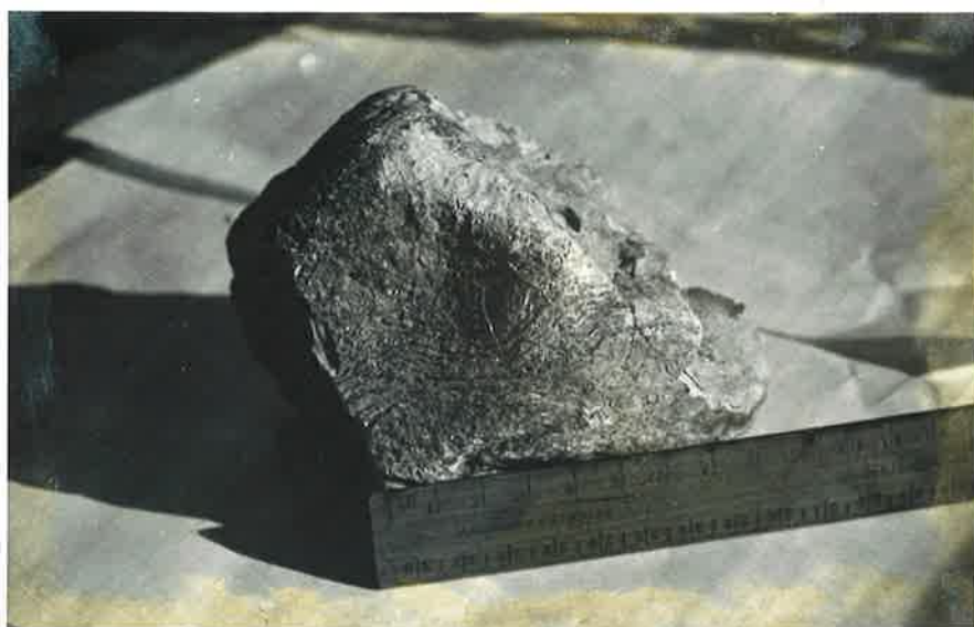
Figure 3.5 Outer surface of strongly indurated hardpan calcrete showing the stromatolitic appearance of the laminar calcrete which surrounds the boulder.
