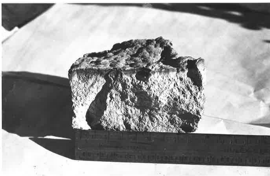
Figure 3.2 Massive hardpan calcrete with a thin horizon of laminar calcrete developed on the upper surface.
