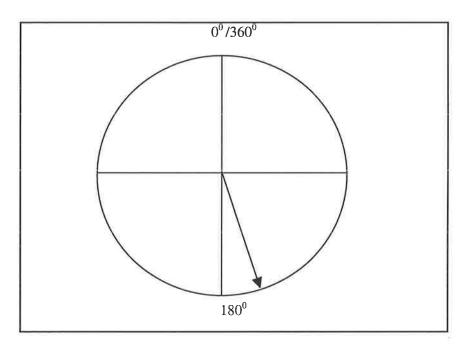
Figure 6.1: Here is an example of an orientation measurement taken from due North. An orientation measurement is an angular value called an azimuth.
