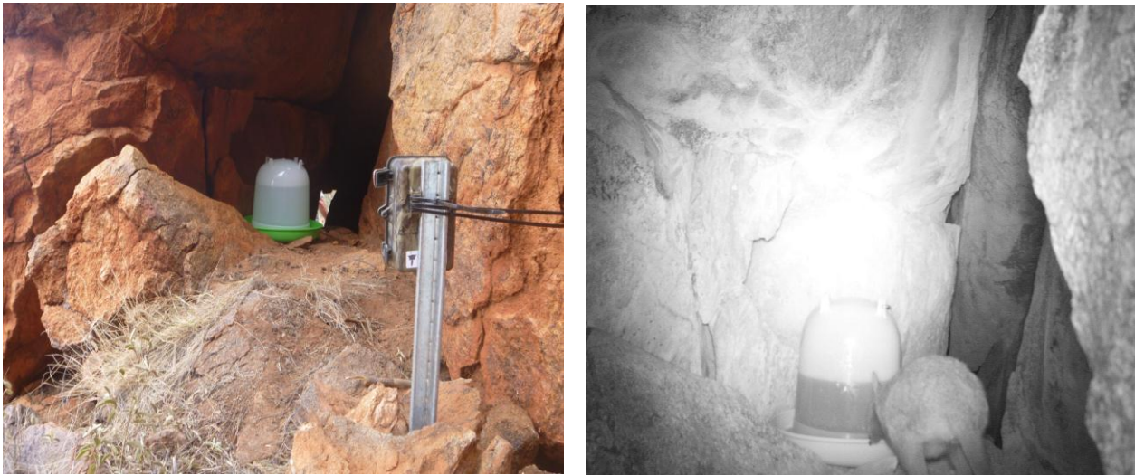
Figure 4.2. Example of the experimental set up used to monitor drinking rates at supplementary water points for wild and reintroduced waru and an exemplar photograph at this point.
