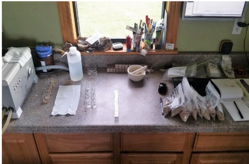
Figure 5.6: Photo of the lab setup while processing samples for magnetic susceptibility and particle size. The machine to the far left is the laser particle sizer used, opposed to the typical way, i.e. hydrometer.
