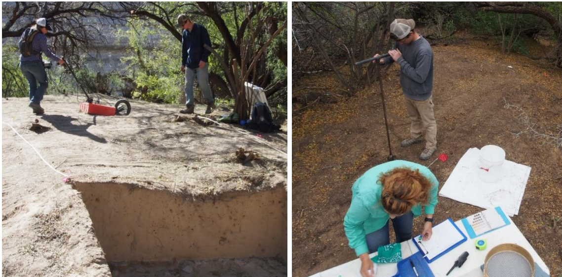
Figure 3.5: (Left) Tiffany Osburn running the GPR across the central grid at Sayles Adobe. (Right) The author and ASWT crewmember Justin Ayers augering in the East Hollow of Sayles.
