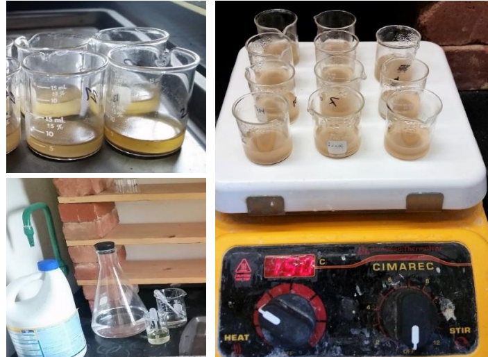
Figure 5.7: (Top left) Samples prior to heating. (Right) Samples heating. (Bottom left) Bleach and sodium hexametaphosphate.
