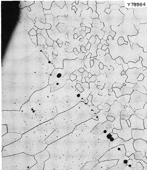
Fig. 16.13. Unalloyed Tungsten Welded with Unalloyed Tungsten Filler Metal. 75 \times . Etchant: \text{NH}_4\text{OH} and \text{H}_2\text{O}_2 . Reduced 32%.
