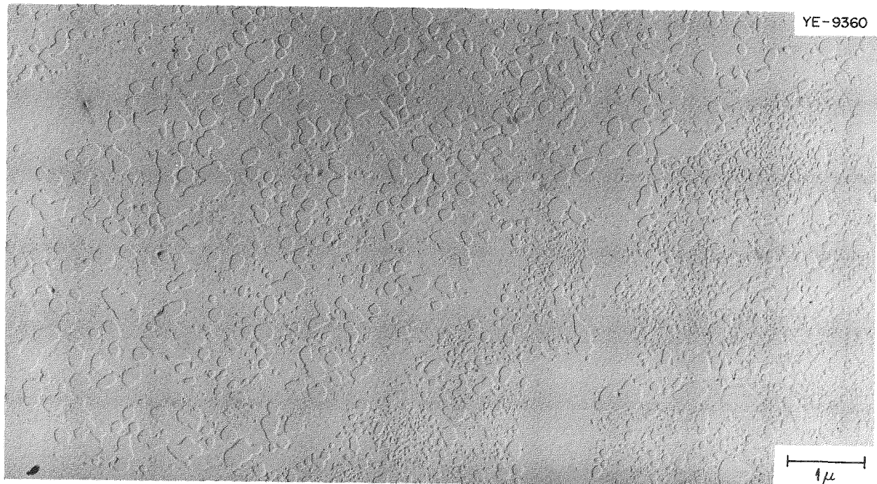
Fig. 19.1. Replica Electron Micrograph of Extruded Rod of Internally Oxidized Modified Nichrome Alloy (Transverse Section).
