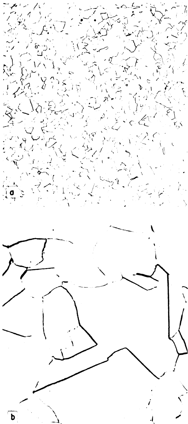
FIGURE 49. Microstructure of high-purity nickel (Nickel 200) as forged. Etched with \text{NaCN} - (\text{NH}_4)_2\text{S}_2\text{O}_8 . a. \times 100 . b. \times 500 .
