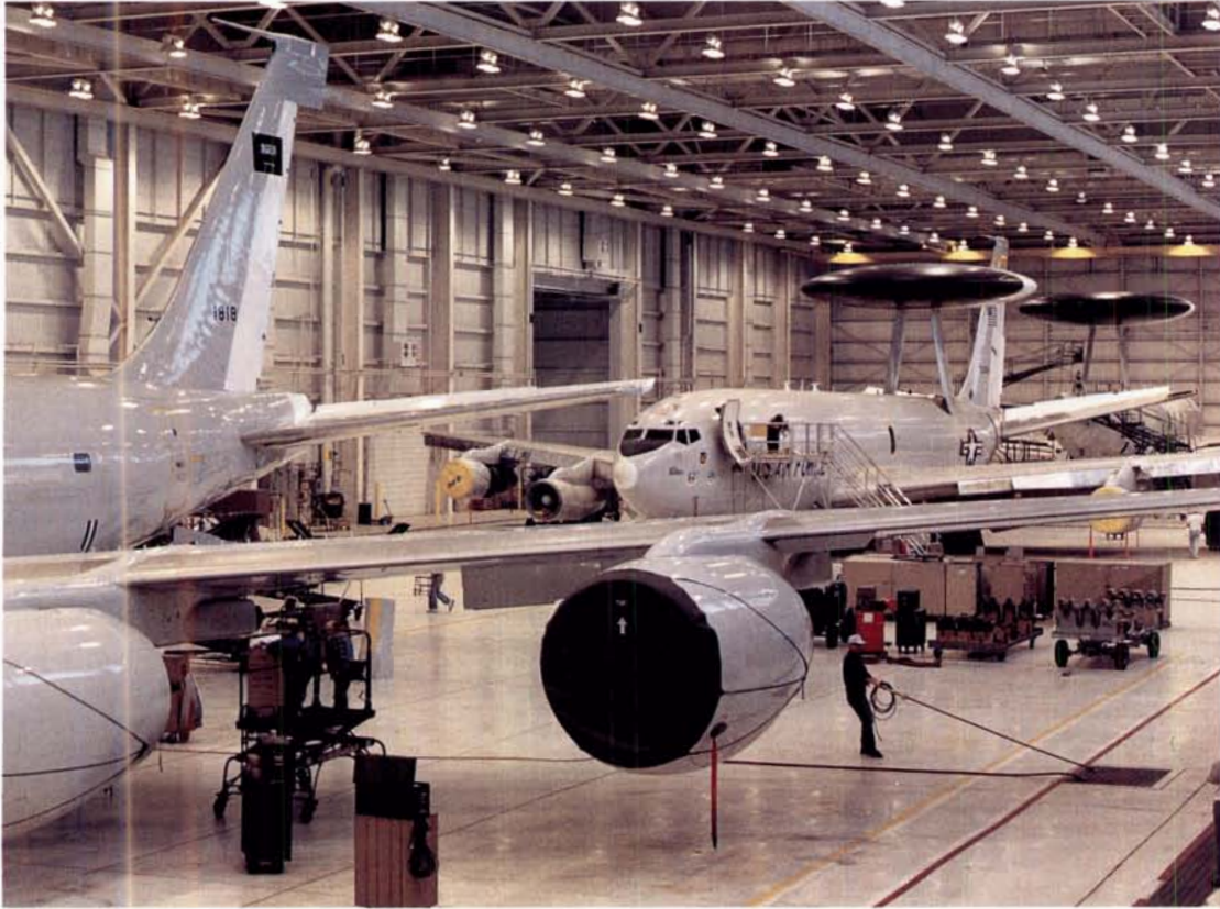
THE CENTER HAS THE ONLY HANGAR IN THE AIR FORCE WITH A SPECIAL HIGH BEAM CEILING TO ACCOMMODATE THE E-3 AIRCRAFT RADAR RADOME.
