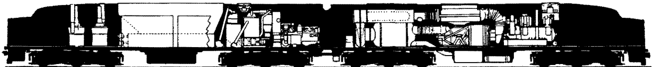
Figure 10. Proposed coal-burning gas turbine locomotive
