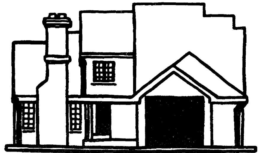
Picture A. What's wrong with his picture? Gutters, downspouts and garage door draw too much attention and give the home an unsettled, choppy appearance.
