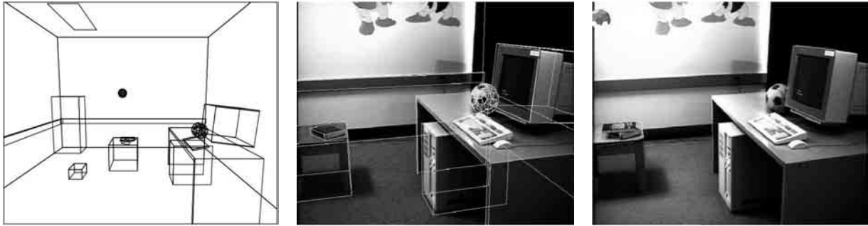
Figure 12: Results for Fournier et al. [FGR93]. Left: wire-frame image, all objects in the scene are represented by a box, that narrowly fits the object. Middle: Image information is mapped on the boxes (note that for the ball, a more complex shape was used). Right: an example of a MR, the book on top of another book, lying on a table is virtual. Also a virtual light source is added. The global common illumination effects are generated with an adaptive progressive radiosity algorithm. Courtesy of Fournier et al.
