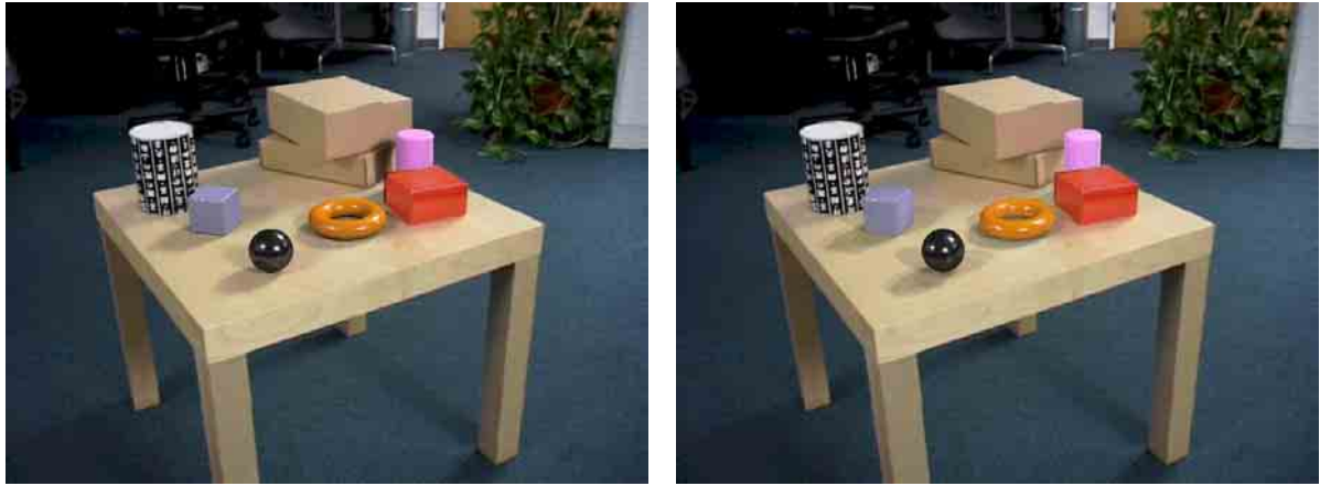
Figure 9: Results for Gibson et al. [GM00]. Comparison of a ray-traced (left) and a hardware generated image (right). The ray-traced image was generated using RADIANCE [War94], the hardware generated image made use of the rendering method described in [GM00]. The generation of the ray-traced image took approximately 2 hours, the generation of the hardware rendered image took place at nearly 10 frames-per-second. Courtesy of Gibson et al.
