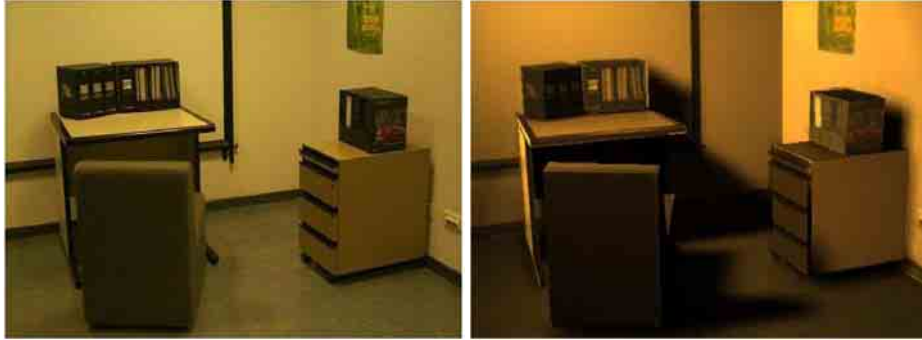
Figure 3: Results for Loscos et al. [LDR00]. The image on the left hand side represents the real scene. The image on the right hand side shows the relighted synthetic scene for which real light sources have been virtually turned off and a virtual light source is inserted. Global common illumination updates are performed at interactive rates using an adapted version of [DS97]. Courtesy of Loscos et al.
