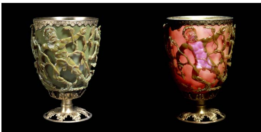
Figure 6. The Lycurgus Cup (British Museum, London) made of dichroic glass, contains colloidal gold and silver that gives its property of being translucent when a light is shone through it.
