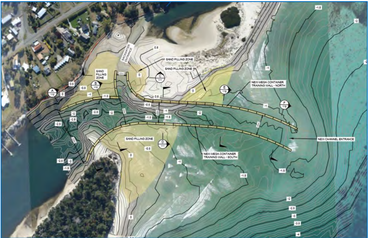
Figure 13, page 42, bottom: Indicative map showing approximate alignment for the northern option for dredging and channelisation, Prosser River, 2017–18. Source: MAST.
