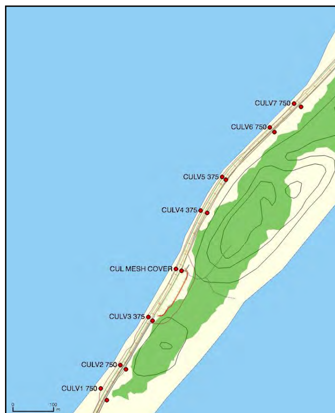
Figure 2: Map showing the Bruny Island Neck colony (green polygon), the Bruny Island Main Road and car park (lower centre), the locations of the eastern (colony) and western (d'Entrecasteaux Channel) entrances of culverts 1 to 7 (south to north) and surface contours (10 m increments). The numbers for each culvert denote their internal diameter (e.g. CULV 1 750: Culvert 1 has 750 mm diameter); contour interval is 10 m and scale bar shows 100 m. Note that it is believed that GPS noise is responsible for the wayward position data for the colony entrance to culvert 1.
