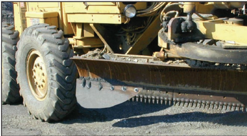
Figure 4.18—Homemade ditch cleaner for a grader.
