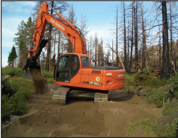
Figure 2.24—Track-laying excavator operates in a sensitive meadow environment with little adverse impact.
