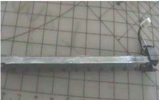
Figure 14 Thin layer of grease on heating element
