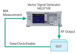
The BER can be measured using the DUT-demodulated Data/Clock/Enable.
