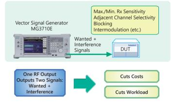
Two modulation signals can be output from one RF output using the baseband signal combine function (MG3710E-048/078). The level ratio (CN = 80 dB) and the frequency offset (±80 MHz max.) can be set as well. Tests using two modulation signals, such as Adjacent Channel Selectivity (ACS), Blocking, and Intermodulation (IM), etc., require two separate signal generators and a license for each, greatly increasing equipment costs and setting work loads.
