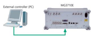
Connect to GPIB, Ethernet or USB port
