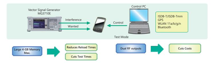
The MG3710E can save up to 1024 Msamples (4 GB) per RF. Memory size is one of the most important specifications for an arbitrary waveform signal generator. Small memory cannot save multiple waveform data and requires time-wasting reloading and measurement to output different signals each time.
