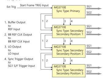
Note: MG3710E-017 is not required when synchronizing the local signal and baseband clock of SG1 (1stRF) and SG2 (2ndRF) installed in one MG3710E unit.
