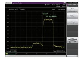
Spectrum of Wanted + Modulated Interference Signals
