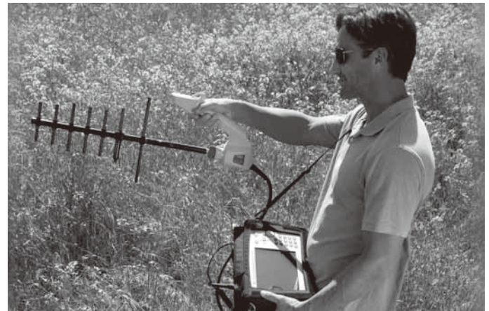
MA2700A Handheld InterferenceHunter with directional antenna and channel filter
