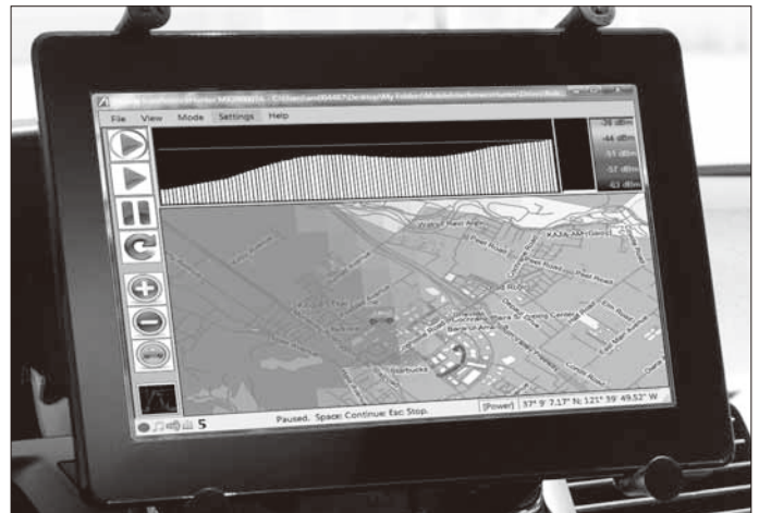
Interference hunt screen capture. Dots shown along drive path are colored according to signal strength.
