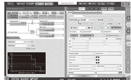
The Help function displays the remote commands corresponding to GUI operations, which simplifies automated system configurations.
