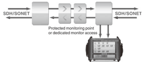
Bi-directional in-service monitoring of SDH/SONET lines
