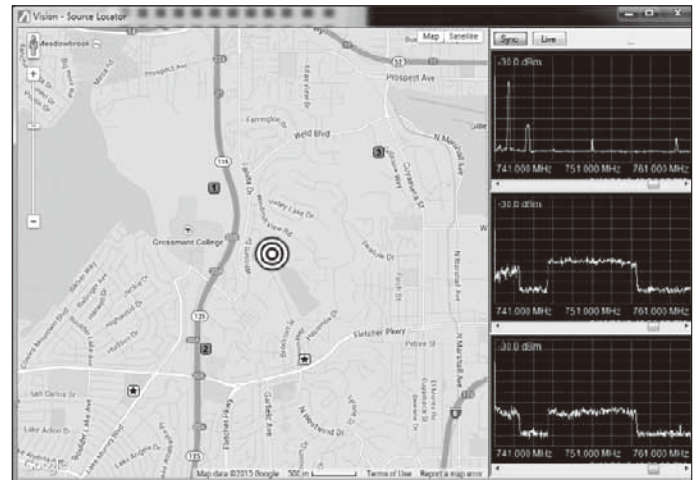
Figure 9: Geo-location of interference position
