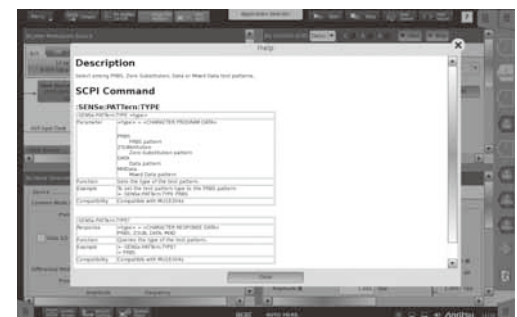
The Help function displays the remote commands corresponding to GUI operations, which simplifies automated system configurations.
