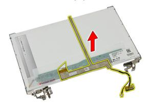
**20.** Remove the screws that secure the display brackets and hinges to the display panel.
