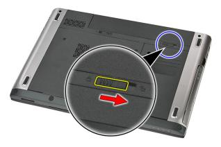
3. Slide the battery and remove it from the computer.
