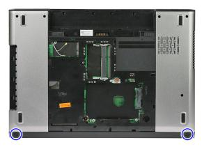
6. Remove the screws that secure the palm rest to the computer.
