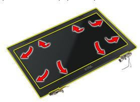
10. Lift up the display bezel and remove.
