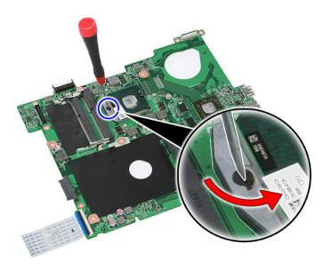
18. Lift up the processor and remove.
