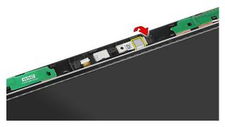
12. Pry the latch, then lift up the display and remove.
