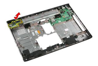
18. Remove the screw that secures the right I/O board.
