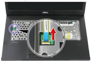
9. Release the touch-pad data cable securing clip.
