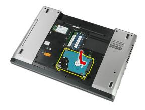
6. Remove the screws that secure the hard-drive bracket to the hard drive.
