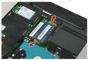
$\textbf{5.} \quad \text{Remove the memory module from its connector on the system board}.$
