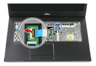
12. Disconnect the quick-launch button board cable.
