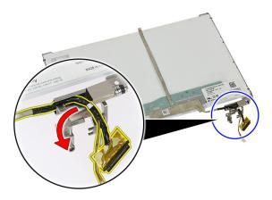
17. Peel open the tape that secures the display cable to the display panel.
