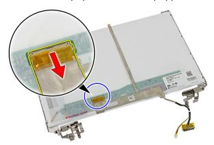
19. Peel off and remove the display cable.
