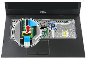
14. Disconnect the fingerprint-reader data cable.
