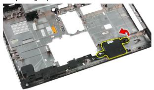
**19.** Release the speaker cables from the routing channel.
