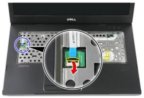
8. Disconnect the power-button board cable.
