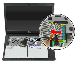
7. If your computer comes with a backlit keyboard, open the keyboard backlight cable securing clip.
