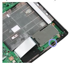
11. Lift up the ExpressCard board at an angle and remove.
