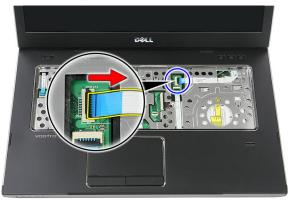
13. Release the fingerprint-reader data cable securing clip.
