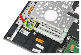
**9.** Release the fingerprint-reader cable from the adhesive affixed to the palm rest.
