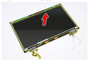
$\textbf{16.} \ \ \text{Release the cables from the left hinge}.$
