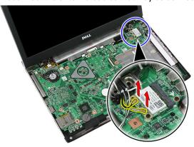
7. Remove the screw that secures the WLAN card.
