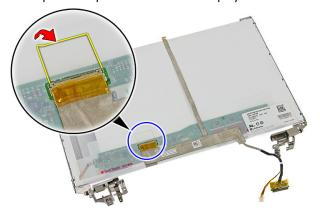
18. Disconnect the display cable from the display panel.
