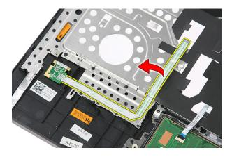
10. Lift up the fingerprint-reader board and remove.
