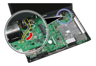
10. Disconnect the display-data cable from the system board.
