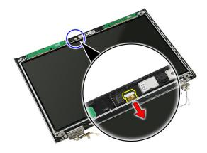
11. Peel off the tape that secures the camera.
