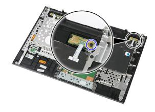
8. Pry the latch to release the power-button board; then lift up and remove.
