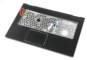
7. Remove the screw securing the power-button board.
