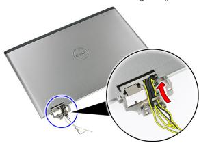
**14.** Remove the screws that secure the display brackets and hinges to the display assembly.
