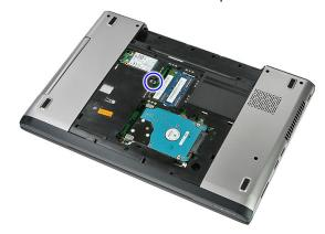
5. Use a screwdriver to nudge the optical drive out of the computer.
