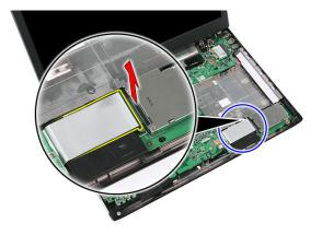
9. Remove the screw that secures the ExpressCard board.
