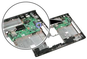
**19.** Lift up the I/O board and remove.
