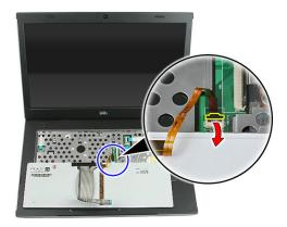
**8.** If your computer comes with a backlit keyboard, disconnect the keyboard backlight cable.
