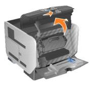
3. Pull the print cartridge up and out of the printer.
