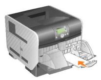
6. Slide the width guide to the left until it lightly touches the stack. Make sure the envelopes do not buckle.
