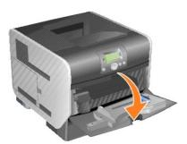
3. Push the release latch to the right to open the top front cover.
