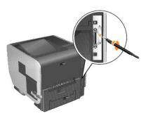
9. Rotate the antenna until the joint allows it to be pointed up.
