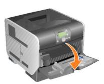
2. Push the release latch to the right to open the top front cover.
