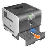
2. Squeeze the side guide tab, and slide the guide to the outer edge of the tray.
