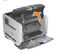
3. Lift and pull the print cartridge out of the printer.
