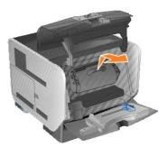
5. Attach the cardboard cover retainer to the hook on the printer.
