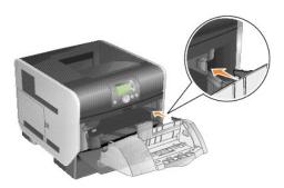
The envelope feeder tilts downward at a slight angle when it is installed properly.
