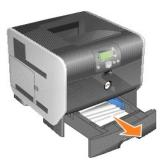
2. Open the duplex tray, and remove the media by pulling up.
