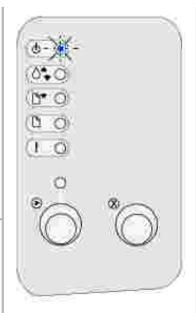
The printer is busy receiving or processing data, or printing a test page. In addition, the toner in the toner cartridge is getting low.
