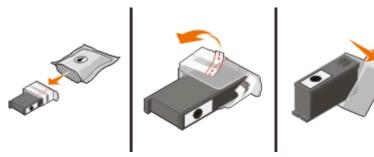
If your ink cartridge comes with a twist cap, then twist and remove the cap.
