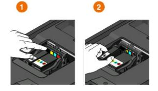
**Warning—Potential Damage:** Do not remove the old cartridges until you have the new cartridges available, or the ink remaining in the printhead may dry out and clog the nozzles.
