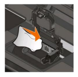
Warning—Potential Damage: Do not touch the printhead ink filter or the printhead nozzles.
