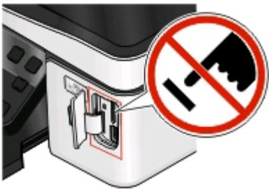
**Warning—Potential Damage:** Do not touch any cables, any network adapter, any connector, the memory device, or the printer in the areas shown while actively printing, reading, or writing from the memory card. A loss of data can occur.
