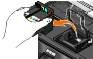
**Warning—Potential Damage:** Do not touch the printhead ink filter or the printhead nozzles.
