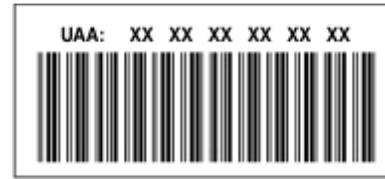
**Note:** A list of MAC addresses can be set on an access point (router) so that only devices with matching MAC addresses are allowed to operate on the network. This is called *MAC filtering*. If MAC filtering is enabled in your access point and you want to add a printer to your network, then the MAC address of the printer must be included in the MAC filter list.
