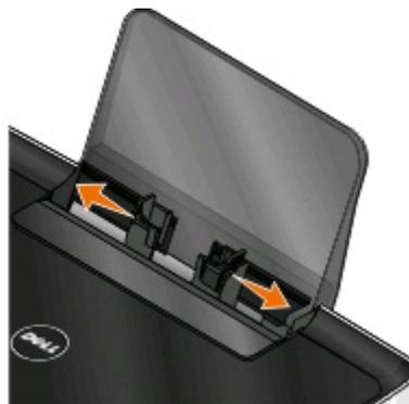
**Note:** Do not force paper into the printer. The paper should be flat against the paper support, and the edges should be flush against both paper guides.
