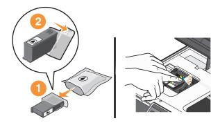
**Note:** Install the ink cartridges immediately after removing the protective cap to avoid exposing the ink to air.
