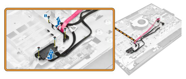
5. Disconnect all the cables that are connected to the system board.
