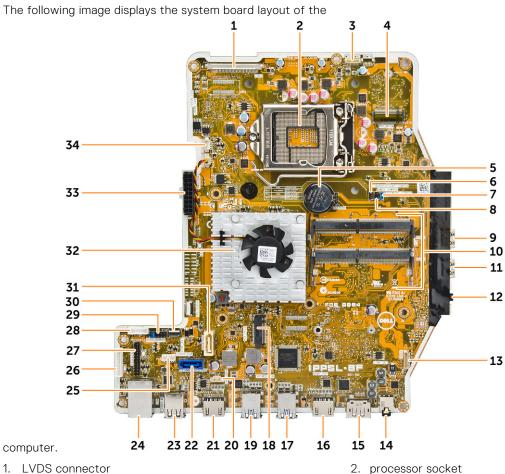
3. camera connector 5. coin-cell battery
