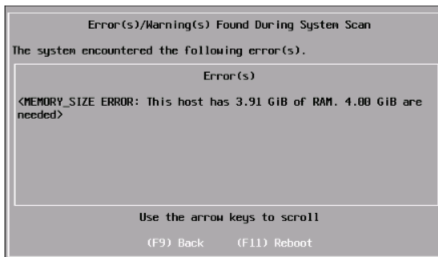
Figure 5. VMware ESXi installation failure
