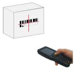
4. Center the symbol in any orientation within the aiming pattern. Ensure the entire symbol is within the rectangular area formed by the brackets in the aiming pattern, then either wait for the timeout or release the scan key to capture the image. A red beam illuminates the symbol, which is captured and decoded.
