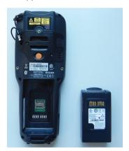
4. Insert the new battery pack into the slot (see Install the Battery on page 7).
