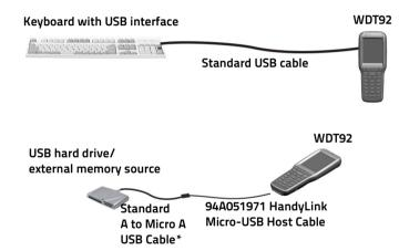
A standard USB cable is needed only if the USB hard driver or flash memory device does not include its own cable with a "A" plug on it.
