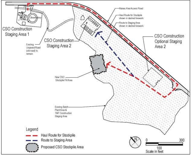
Figure 4-1: Conceptual Plan View of Overall Deconstruction Staging
