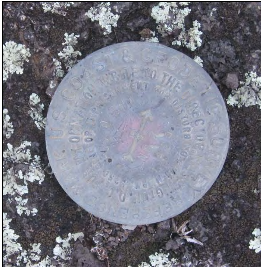
Figure 78. One of several geodetic datum markers beneath and around triangulation station, view to east
