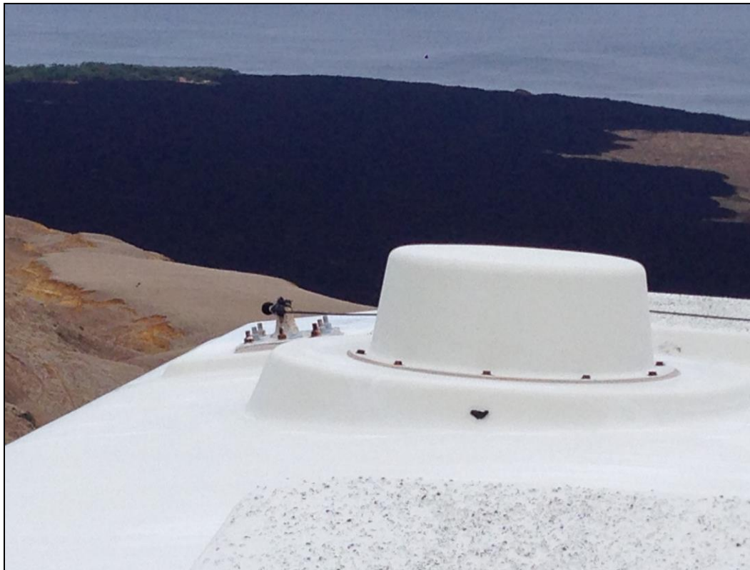
Figure 2. Bat detector microphone mounted on nacelle.
