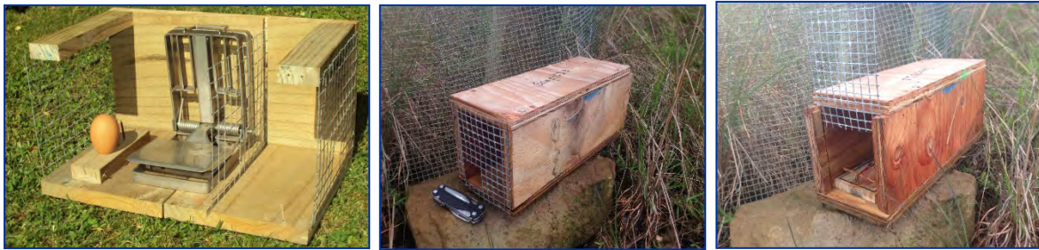
Figure 11.1. Bird Excluding Box for DOC 200 Snap Traps from Makamaka'ole Project, Maui
