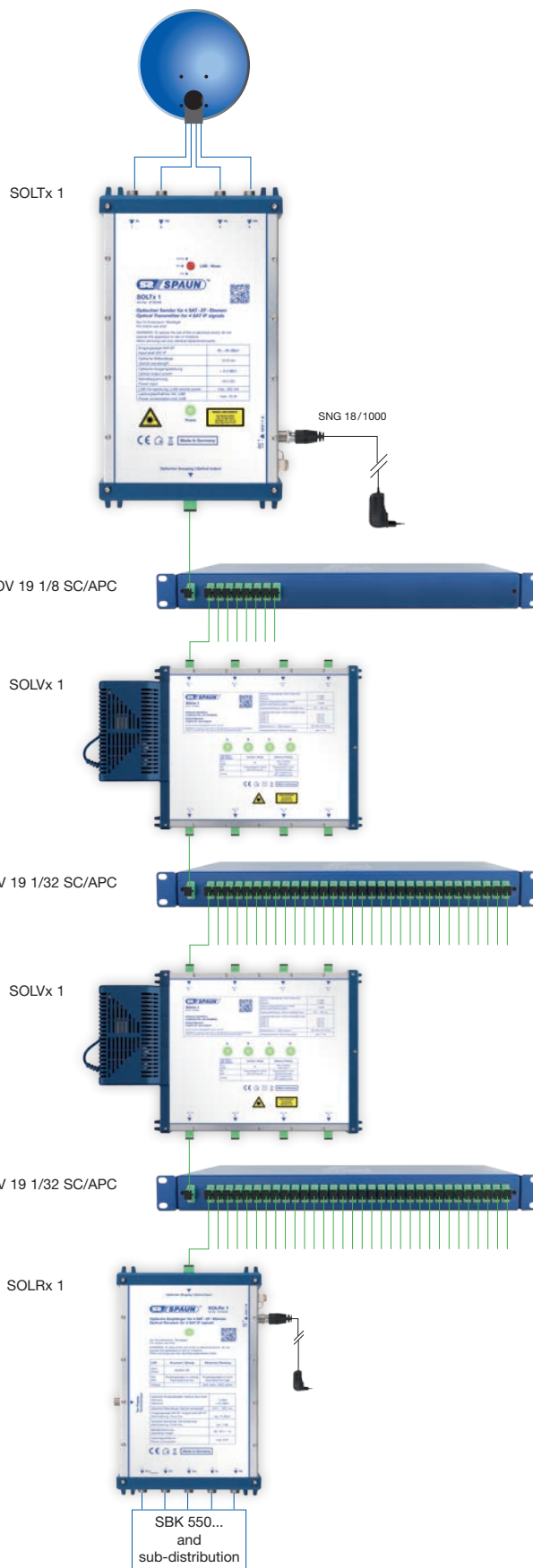
Optical distribution of 4 SAT IF signals to up to 8192 optical nodes with subsequent sub-distribution.
