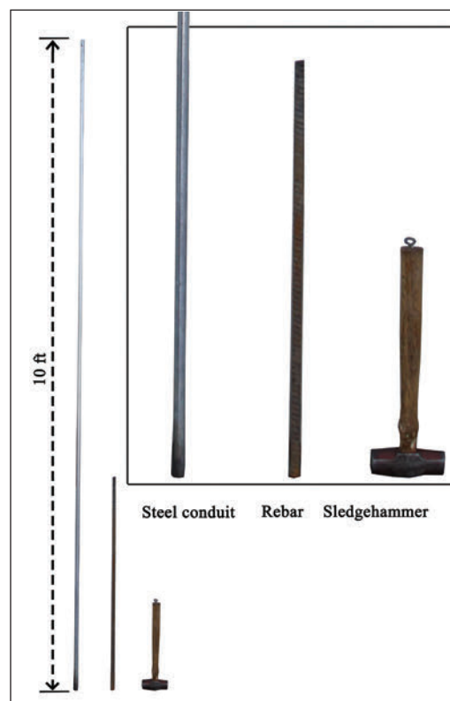
Figure 7. Materials for suspending traps: steel conduit (EMT), rebar, and a sledgehammer.
