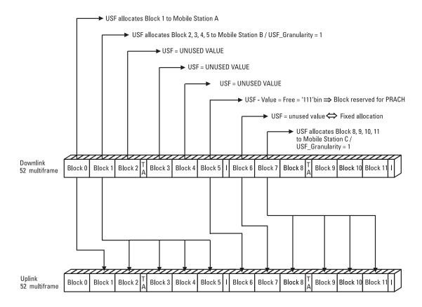
Figure 3.30 Example of the operation of the USF on a time slot with PCCCH and fixed allocation.
