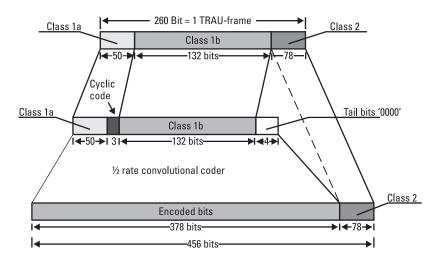
Figure 1.23 The process of convolutional coding for FR speech.
