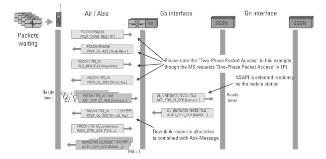
Figure 4.18 A mobile originating PDP context activation via the PCCCH.
