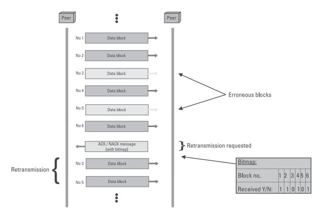
Figure 5.5 The procedures of BEC aided by ARQ.
