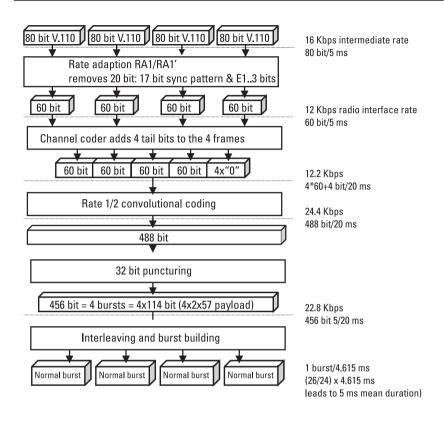
Figure 6.8 80 TCH/F9.6, V.110 frame air interface.
