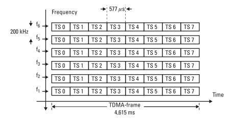
Figure 1.11 The combination of FDMA and TDMA in GSM.
