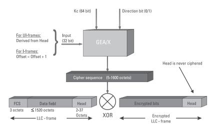
Figure 5.17 The process of encryption in GPRS/LLC.
