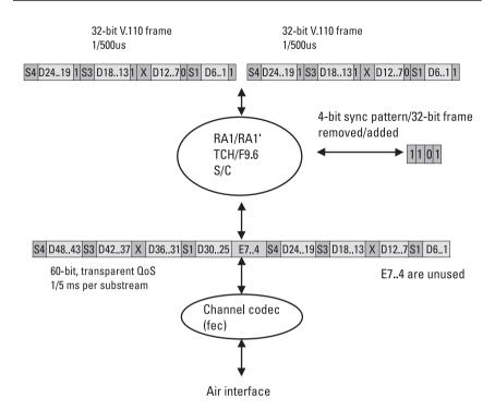
Figure 6.27 RA1/RA1', TCH/F9.6, 48 Kbps, synchronous.
