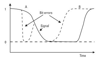
Figure 1.25 Single and multiple bit errors at the receiver.
