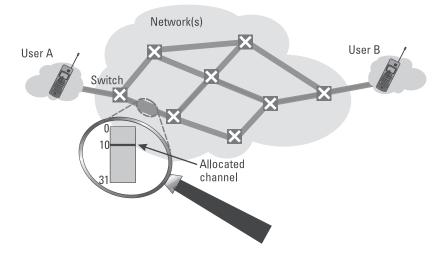
Figure 2.4 The principle of circuit switching.
