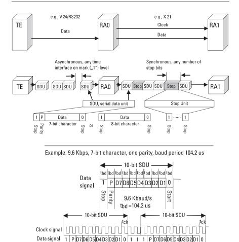
Figure 6.20 RA0 serial data units.
