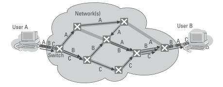
Figure 2.5 The principle of packet switching.
