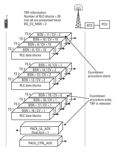
Figure 3.35 Example of the countdown procedure on one time slot.
