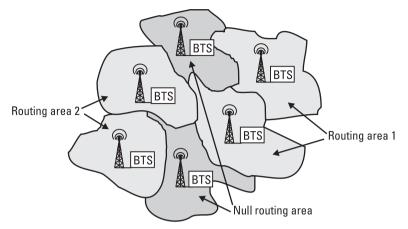
Location area = routing area 1 + routing area 2 + null routing area
