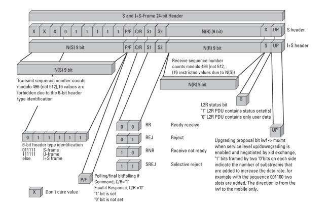
Figure 6.39 S, I + S-frame header.
