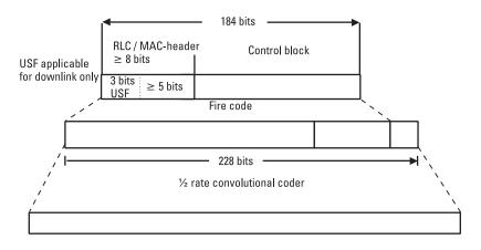
Figure 3.16 CS-1 in the coding of RLC/MAC control messages.
