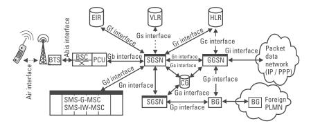
Figure 2.23 Interfaces between the GSM and the GPRS network elements.
