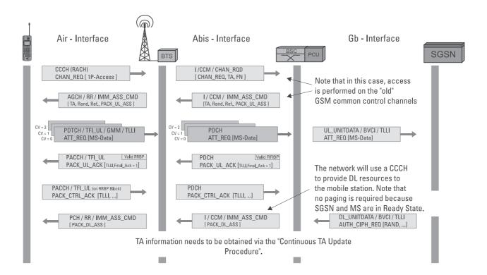
Figure 4.6 The GPRS attach via the CCCH.
