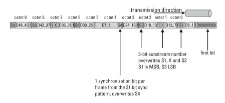
Figure 6.5 80-bit V.110 mapping, frame sync pattern, and subchannel number.
