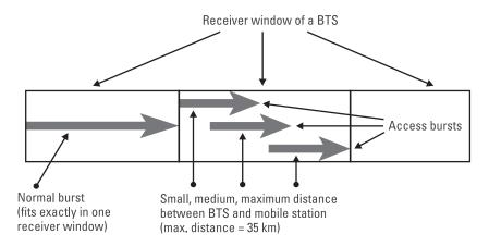
Figure 1.14 The short length of the access burst allows it to be sent from distances of up to 35 km.
