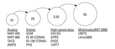
Figure 2.1 Mobile communications generations 1 to 3.
