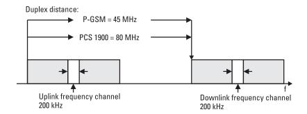
Figure 1.9 There is a set distance between the uplink and downlink channels in the application of FDMA in GSM.
