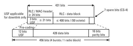
Figure 3.18 Coding according to CS-4.
