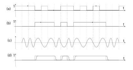
Figure 1.35 The path from FSK to GMSK: (a) Bit stream, (b) bit stream after XOR operation, (c) MSK signal, and (d) behind Gaussian filter.
