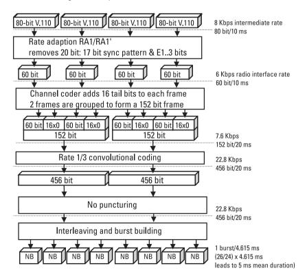
Figure 6.9 TCH/F4.8, V.110 frame air interface.
