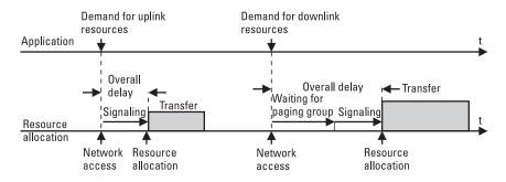
Figure 2.11 Delay times in resource allocation in uplink and downlink directions.
