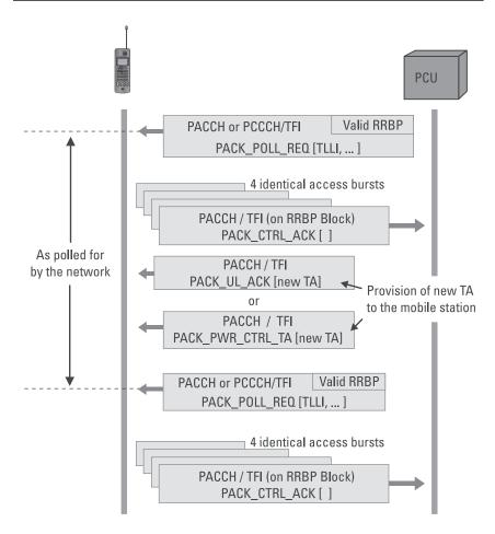
Figure 3.13 The use of polling as an alternative to the determination of the timing advance.
