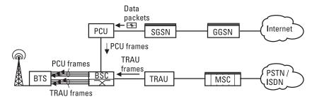
Figure 2.15 Conversion of packet data into PCU frames by the PCU.
