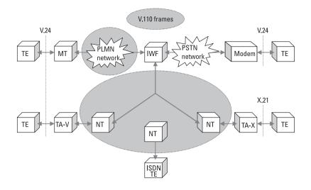
Figure 6.13 V.110 in ISDN and GSM PLMN.
