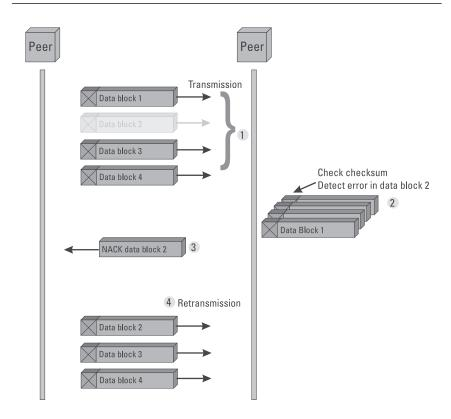
Figure 5.4 The disadvantages of BEC.
