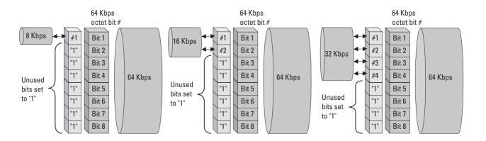
**Figure 6.22** RA2, octet filling, intermediate rate  $\Leftrightarrow$  64 Kbps.
