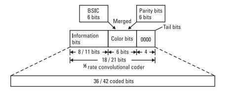
Figure 1.32 The convolutional coding of access bursts.
