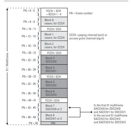
Figure 1.18 Example of a 51 multiframe with a duration of 235.38 ms in the downlink direction of time slot 0 of a BCCH carrier.
