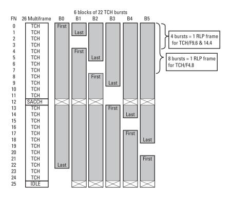
Figure 6.24 Synchronization of V.110 multiframe (RLP-Frame) and TDMA multiframe.
