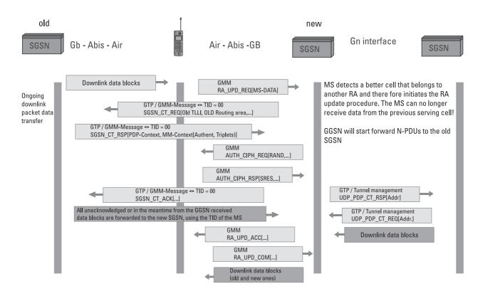
Figure 4.12 Routing area update with SGSN change during data transfer.
