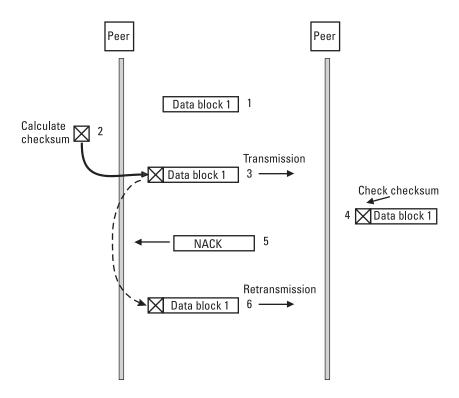
Figure 1.22 The processes of BEC.
