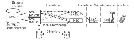
Figure 1.38 The transmission of short messages in a combined GSM/GPRS network.
