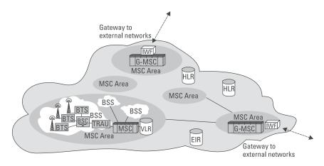
Figure 1.1 GSM network architecture.
