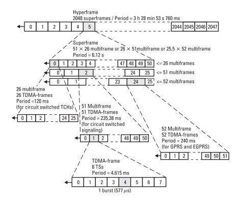
Figure 3.1 The GSM frame hierarchy with the 52 multiframe for GPRS.
