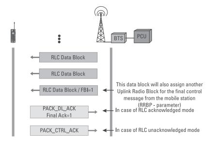
Figure 3.33 The termination of a downlink TBF via the FBI bit.
