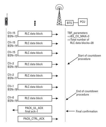
Figure 3.36 Example of the countdown procedure on four time slots.
