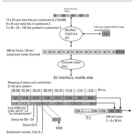
Figure 6.28 RA1/RA1', TCH/F14.4, 48 Kbps, synchronous.
