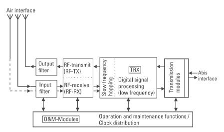
Figure 1.2 Principal schematic diagram of the base transceiver station.
