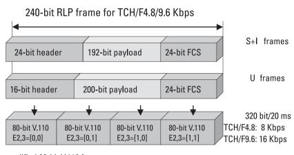
modified 80-bit V.110 frames, not modified: 17-bit sync pattern, E1..E3, D1..D48 modification: D'1..D'12 replacing S, X, E4..7 bits
