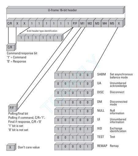
Figure 6.38 U-frame header.
