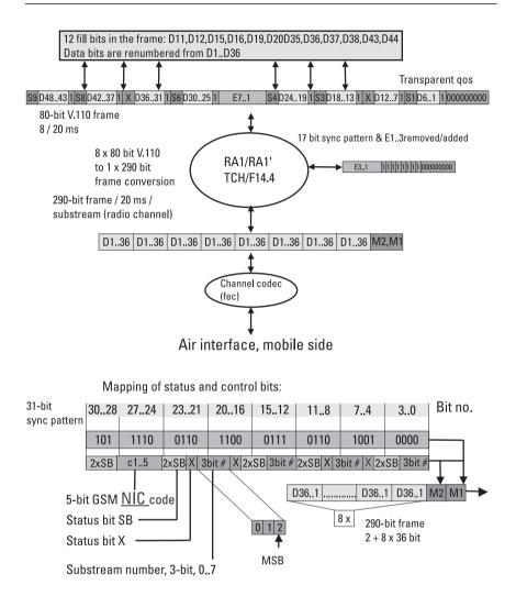
Figure 6.26 RA1/RA1', TCH14.4, data rate < 38.4 Kbps.
