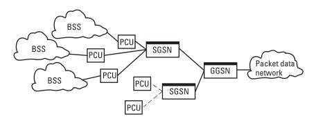
Figure 2.16 The positioning of the SGSN in the network as a whole.
