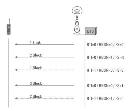
Figure 5.11 The function of RBSN in conjunction with the RTI field and FS bit.
