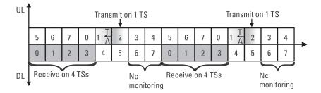
Figure 2.24 Example of the operation of a multislot class 12 with neighboring cell level measurements, taking timing advance into account. The mobile station receives on four time slots and transmits on one.
