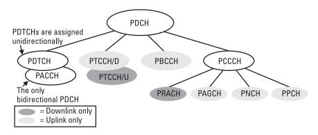
Figure 3.4 The various packet data channels and their directional dependence.
