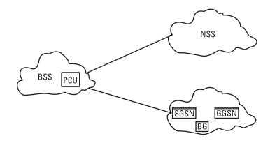
Figure 2.13 The BSS is used equally by the NSS and the GPRS core network.
