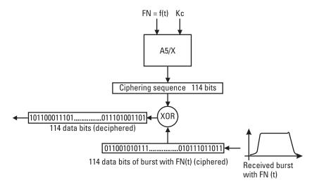
Figure 1.28 The process of deciphering in GSM.
