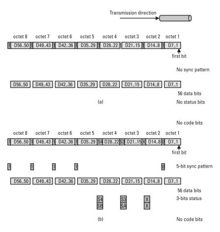
Figure 6.17 64-bit V.110 frame: (a) basic and (b) alternative.
