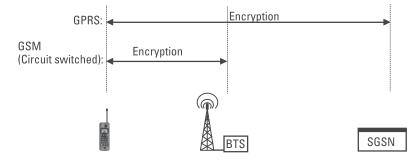
Figure 2.17 The encryption function in GSM and GPRS.
