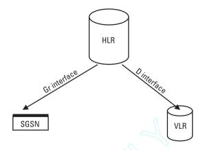
Figure 4.1 The HLR as a mutual basis for SGSN (GPRS) and VLR (GSM).
