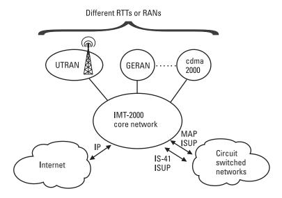
Figure 2.3 A fully developed 3G network with various radio access networks/radio transmission technologies (RTTs).
