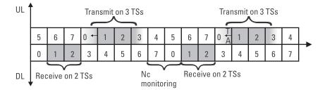
Figure 2.25 Example of the operation of a multislot class 12 with neighboring cell level measurements, taking timing advance into account. The mobile station receives on two time slots and transmits on three.
