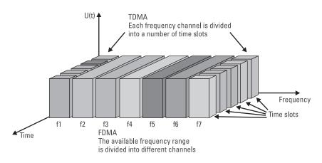
Figure 1.10 The combination of FDMA and TDMA.
