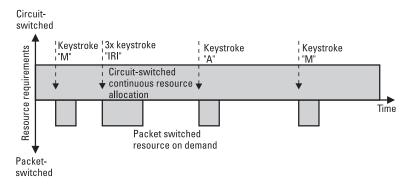
Figure 2.6 Example of a Telnet session, once circuit switched and once packet switched.
