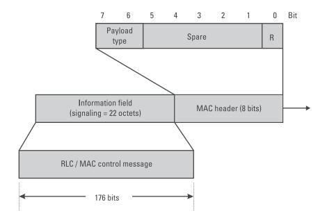
Figure 5.10 The format of the RLC/MAC frame for uplink transfer of RLC/MAC control messages.
