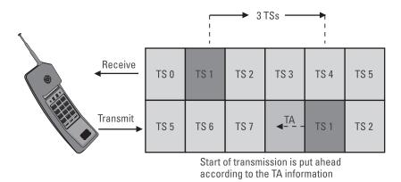
Figure 1.13 The mobile station sets its start of transmission ahead according to the timing advance.
