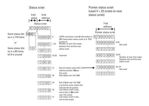
Figure 6.46 L2R-BOP PDU: status octet and pointer status octet.
