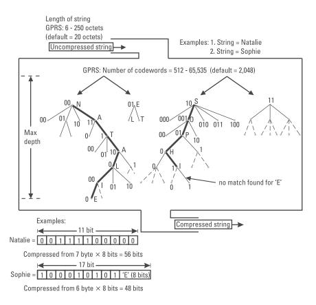
Figure 2.18 Principles of V.42bis compression.
