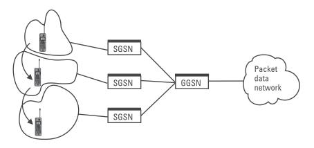
Figure 2.20 The anchor function of the GGSN.
