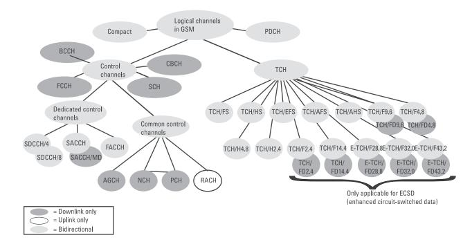
Figure 1.16 The logical channel types in GSM.
