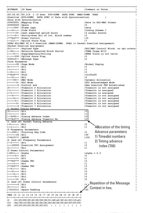
Figure 3.10 Example of a PACK\_DL\_ASS message with allocation of a PTCCH/U subchannels to time slot 2.
