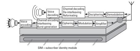
Figure 1.7 Circuit diagram of a GSM mobile station.
