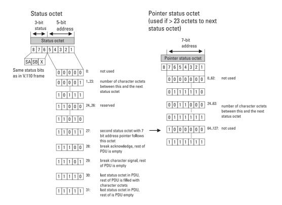
Figure 6.43 L2R-COP PDU: status octet and pointer status octet.
