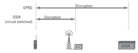
Figure 5.18 The range of encryption in GSM and GPRS.
