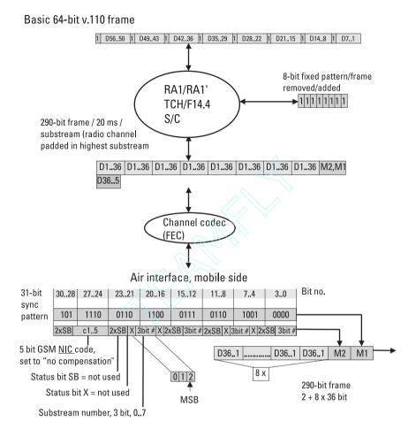
Figure 6.30 TCH/F14.4, 56 Kbps, synchronous.
