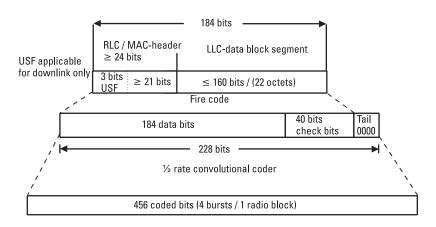
Figure 3.15 CS-1 in the coding of LLC data.
