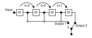
Figure 1.24 Example of a 1:2-rate convolutional coder.
