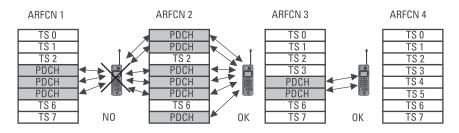
Figure 3.6 GPRS resources can only be occupied on one ARFCN.
