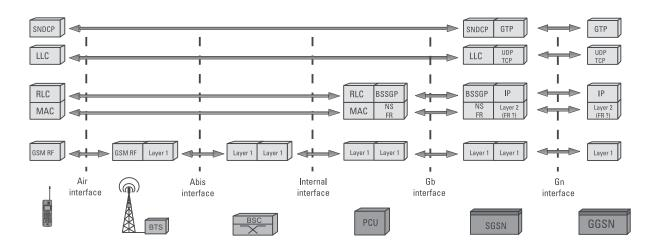
Figure 5.1 Overview of the GPRS protocol stack.
