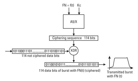
Figure 1.27 The process of data encryption in GSM.
