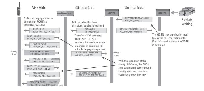
Figure 4.19 A mobile terminating PDP context activation via the PCCCH.
