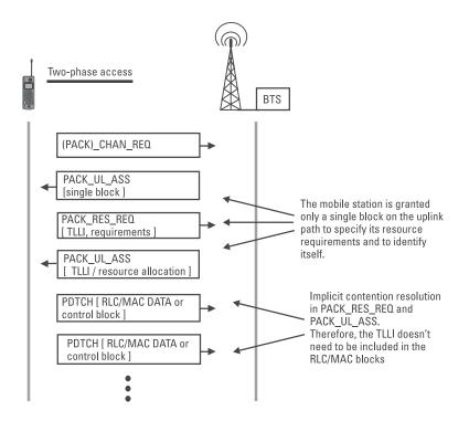
Figure 3.23 The procedures of two-phase packet access (CCCH and PCCCH).
