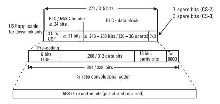
Figure 3.17 Channel coding according to CS-2 and CS-3.
