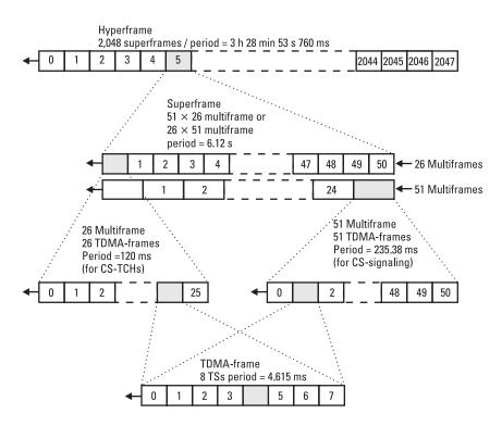
Figure 1.20 The frame hierarchy in GSM.
