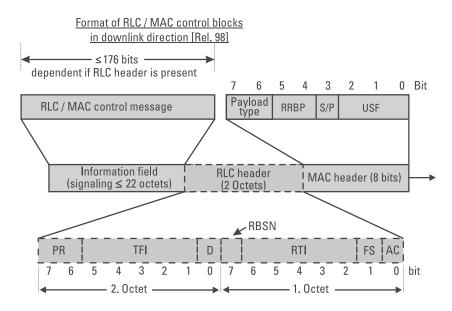
Figure 5.9 The format of the RLC/MAC frame for downlink transfer of RLC/MAC control messages.
