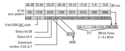
Figure 6.6 290-bit frame mapping, frame sync pattern, and subchannel number.
