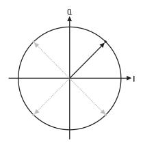
Figure 1.36 GMSK on the I/Q level.
