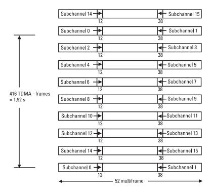
Figure 3.9 The definition of the 16 PTCCH/U subchannels.
