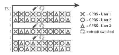
Figure 3.3 Example of resource sharing of GSM and GPRS on an ARFCN.
