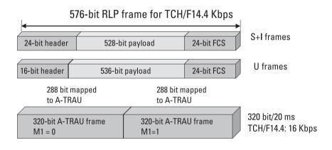
Figure 6.37 RLP frame setup and V.110/A-TRAU mapping.
