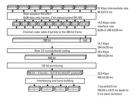
Figure 6.10 TCH/F14.4, V.110 frame air interface.
