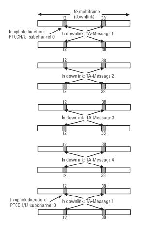
Figure 3.12 Transmission of the new timing advance values in the timing advance messages.
