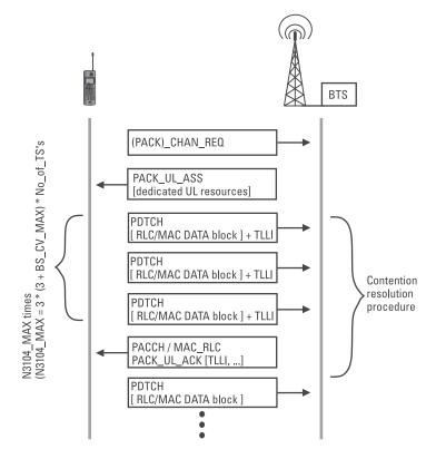
Figure 3.22 The procedure of one-phase packet access (CCCH and PCCCH).
