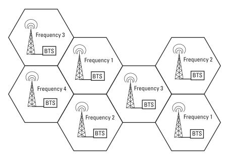
Figure 1.8 The SDMA multiple access process gives rise to cellular network architecture.
