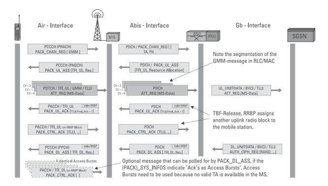
Figure 4.7 The GPRS attach via the PCCCH.
