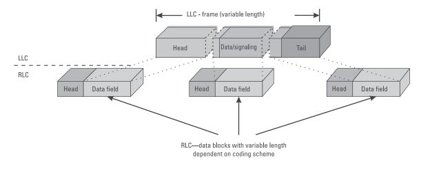
Figure 5.3 The segmenting of LLC frames by RLC.
