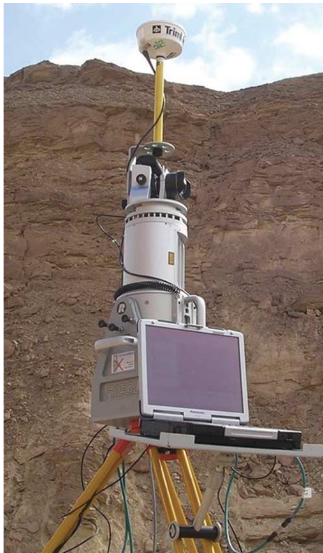
Fig. 4. The fully integrated scan unit (LiDAR, Nikon D100, laptop and DGPS) mounted on the tilt mount and surveyor's tripod.
