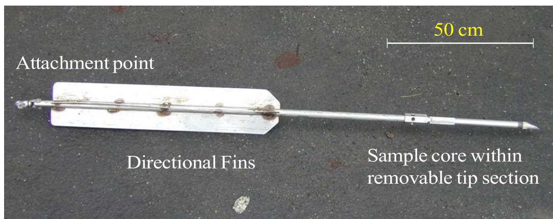
Figure 6: Javelin corer
